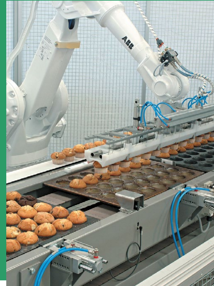
Mechatronics-based industrial manufacturing equipment controlled by a processor in accordance with the set program with no human participation
